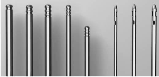
Fig. 7.4 VASER® probes and cannulae. VASER® probes have a different number of rings to efficiently emulsify fat of varying degrees of fibrousness: 3-ring probe for soft fat, 2-ring probe for moderate fat, 1-ring probe for hard fatty or fibrous tissue. The “SST” cannulae used with the VASER® system have smaller holes than other cannulae. The surface area of the holes allows improved efficiency while minimizing trauma during aspiration
